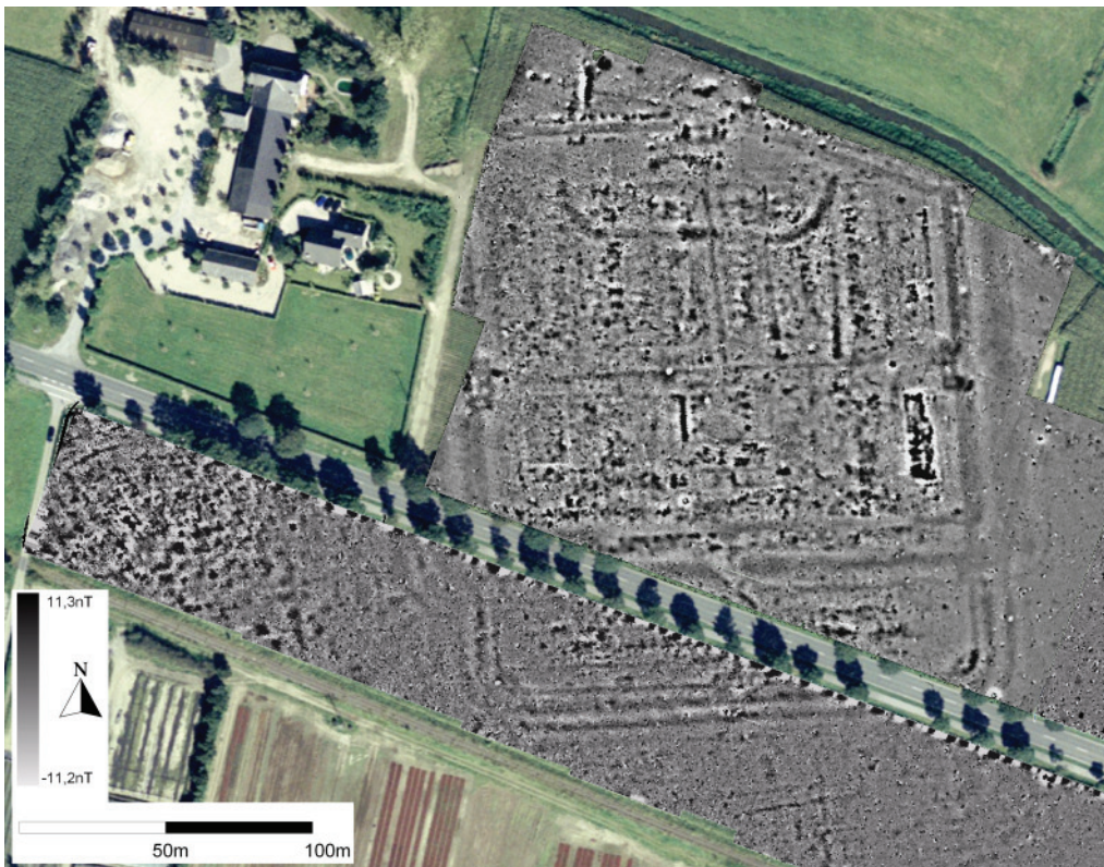
Aerial view with projection of geomagnetic survey of the fort of Burginatium/Altkalkar (Germany).
